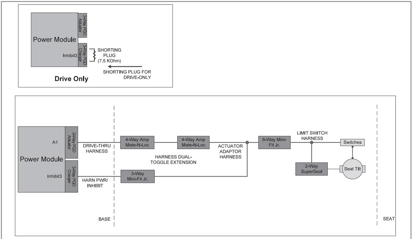
**PM DRIVE ONLY AND THRU-DRIVE ACTUATOR CONNECTIONS**
