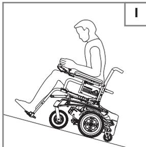
**NOTE**– The solid state controller of your chair has a logic system that will help control your speed when driving on a slope or uphill.
