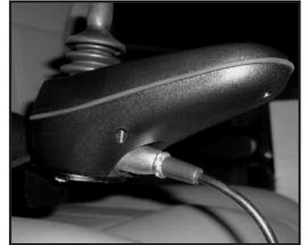
**Off-board charger port (located under joystick)**
