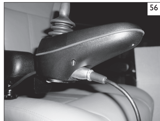
Off-board charger port located under joystick
