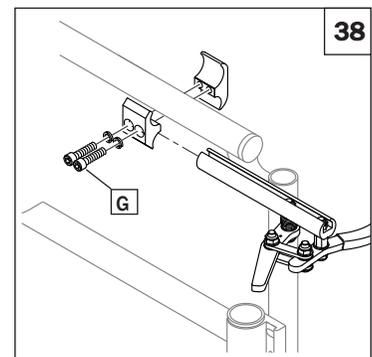
**NOTE-** Clamp and wheel lock may need to be rotated to clear frame tubing.
