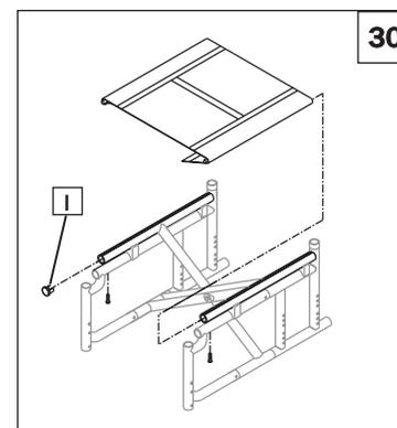
**Q. SIDE GUARDS** 31**Inserting and Removing the Side Guard**
