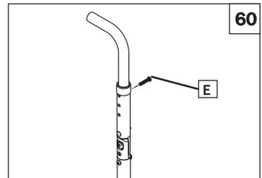
**NOTE-** Use a torque setting of 144 in-lbs when adjusting backrest.
