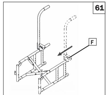
When adding an after-market back, the back canes can be moved forward or rearward by repositioning the backrest pivot plate (F) in the predrilled holes on the frame.
