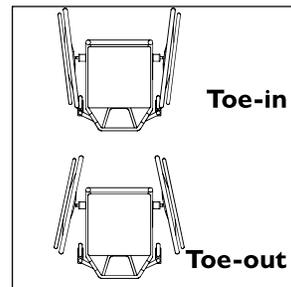
To check that the rear wheels are properly aligned, measure the centerline to centerline of the tires at the midpoint front and rear until the desired measurement is achieved.
