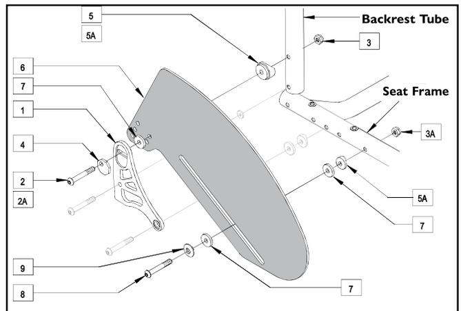
**Figure A – Folding Back, Zero Offset****FOLDING BACK- 1/4-in OFFSET (FIG. B)**
