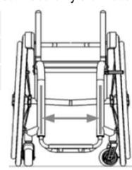
To find the distance between the centerlines of the front frame tubes, **measure the wheelchair directly** if possible. If the chair is not available, you can calculate this distance for either rigid or folding frames by **subtracting the inset** from each side of the seat width, then **subtracting the frame tube diameter**.
