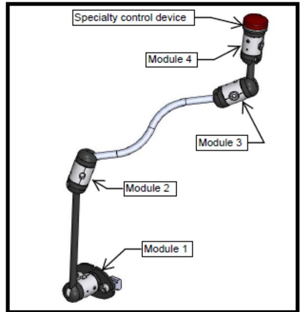
This configuration is not ok. Four (4) modules have been used in sequence going to only one (1) specialty control.
